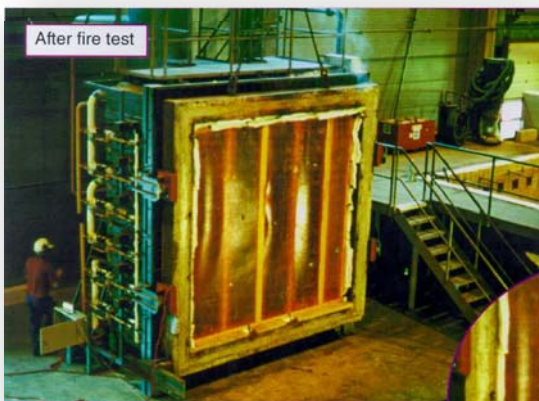
Image After 2 hours fire load in the test rig at Norwegian Fire Laboratory,.
