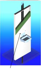
All water installation is hidden inside the wall . Figure tape on the BEET sandwich surface indicate where the faucet is.
